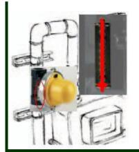
Install using the appropriate level control chain, which should be centered on the check ring when the valve is in the most favorable position
