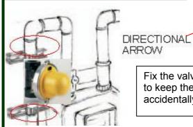
Fix the valve firmly with a fixing bracket to keep the valve from triggering
