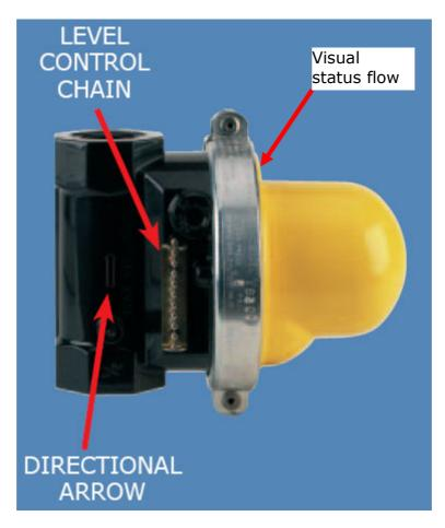
These valves are earthquake sensitive gas shut-off valves. They are intended to close in the event of an earthquake to prevent gas flow into a structure where earthquake damage may have occurred. The valve reduces the potential for fire or explosion due to the release of natural gas into a structure where gas lines, gas fixtures, or gas appliances.
